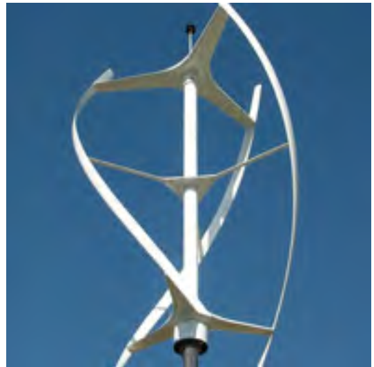
Figure 12: Quiet Revolution twisted Darrieus wind turbine
